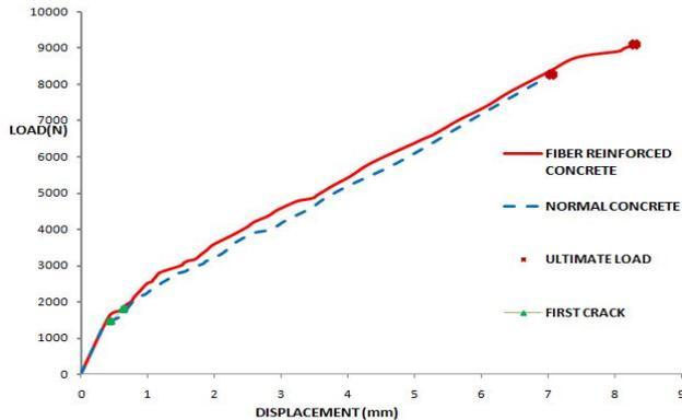
Fig. 12: Typical Load-Displacement Graph.
