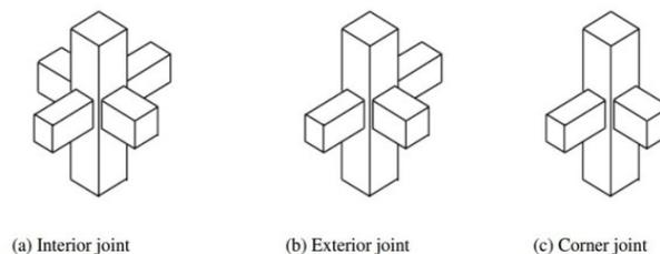
Fig. 1: Types of beam-column joints [Uma and Prasad, 2006]
