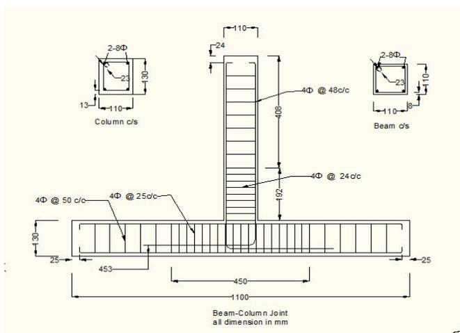
Fig. 2: Detailing of Beam-Column joint
