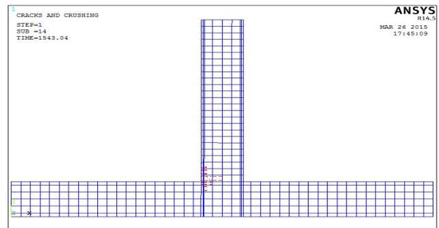
Fig. 6: First crack in Normal Concrete
