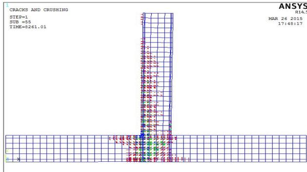
Fig. 7: Ultimate cracks for Normal Concrete
