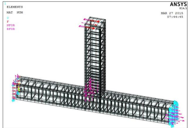
Fig. 5: Finite element model of Normal Concrete and Fiber Reinforce Concrete
