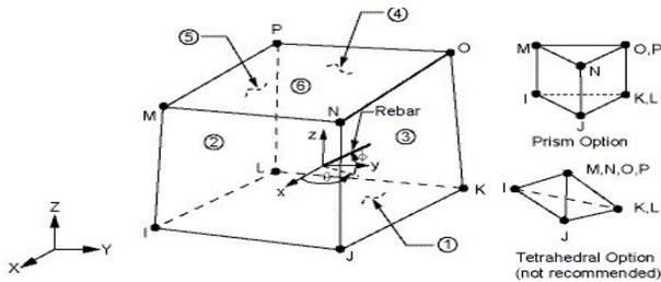
Fig. 3: SOLID65 Geometry
