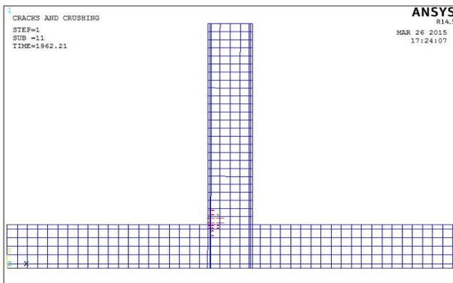
Fig. 9: First crack in Fiber Reinforced Concrete
