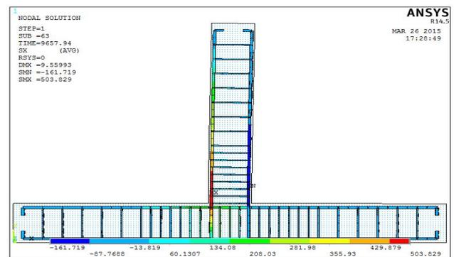
Fig. 11: Ultimate failure load and ultimate stresses for Fiber Reinforced Concrete
