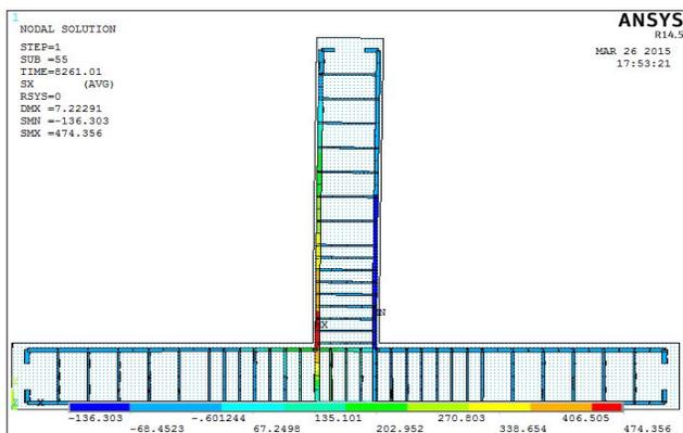
Fig. 8: Ultimate failure load and ultimate stresses for Normal Reinforced Concrete
