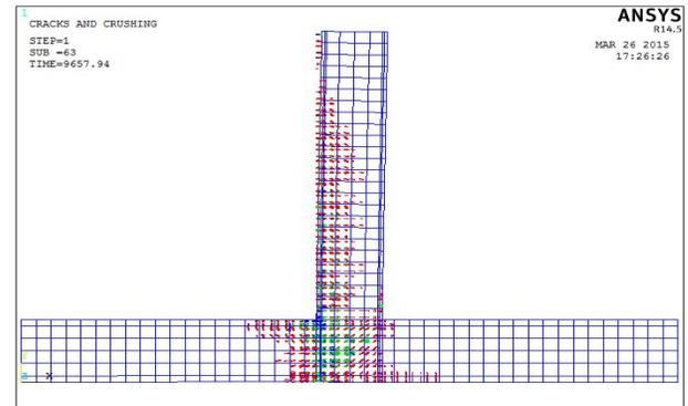
Fig. 10: Ultimate cracks for Fiber Reinforced Concrete
